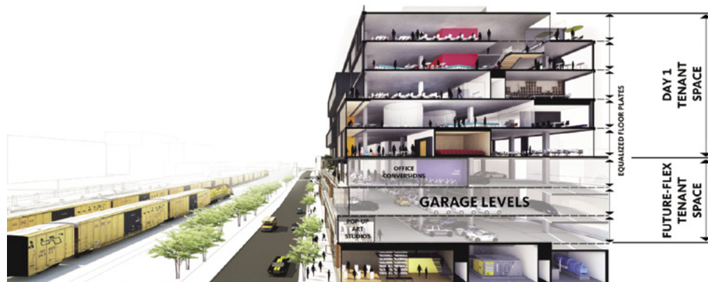
Giambrocco, a mixed-use project in Denver, includes three floors of flexible garage space that can be converted into office space. Credit: Gensler
