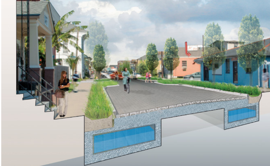
This illustration from the Greater New Orleans Urban Water Plan shows how redesigning streets with elements like rain gardens and pervious pavement can help slow and store stormwater. Credit: Waggonner & Ball.
