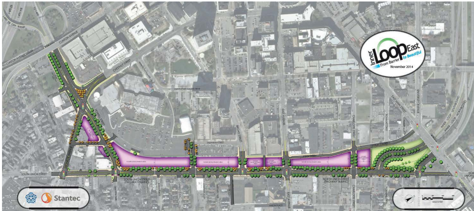
To convert a sunken highway to an at-grade boulevard, Rochester demolished retaining walls and bridges and imported 120,000 cubic yards of dirt. Credit: City of Rochester/Stantec.
