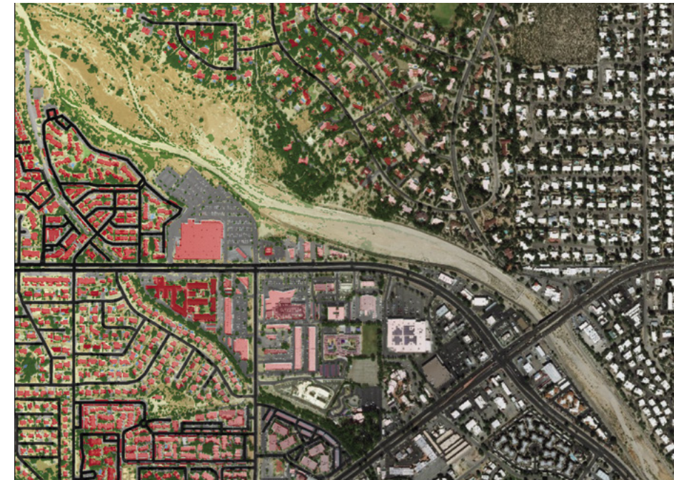
Chesapeake Conservancy's high-resolution land cover data—shown here beside the source imagery used to produce it—accurately depicts small features across the landscape. This level of detail is critical for planning projects that work with individual properties and landowners. Credit: Conservation Innovation Center
