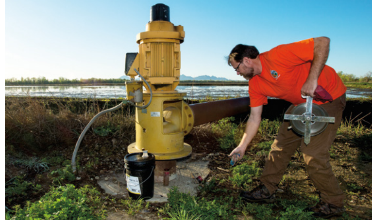
As part of California’s effort to monitor groundwater levels, a state geologist measures the water depth at an agricultural well in the Central Valley. Credit: Kelly M. Grow/California Department of Water Resources.
